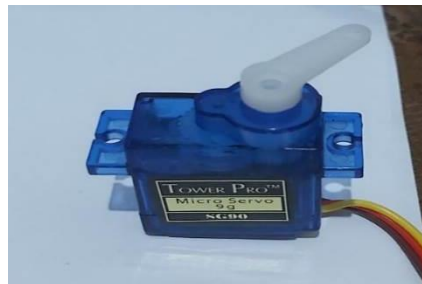
Figure 8. Servo motor at the moment of not moving position at an angle of 0 degrees
