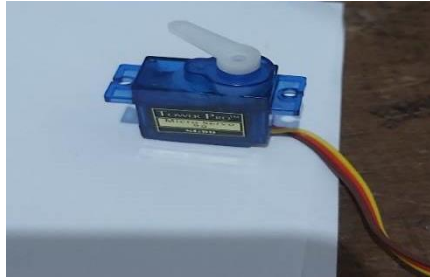
Figure 9. Servo motor at the time of moving position at an angle of 85 degrees
